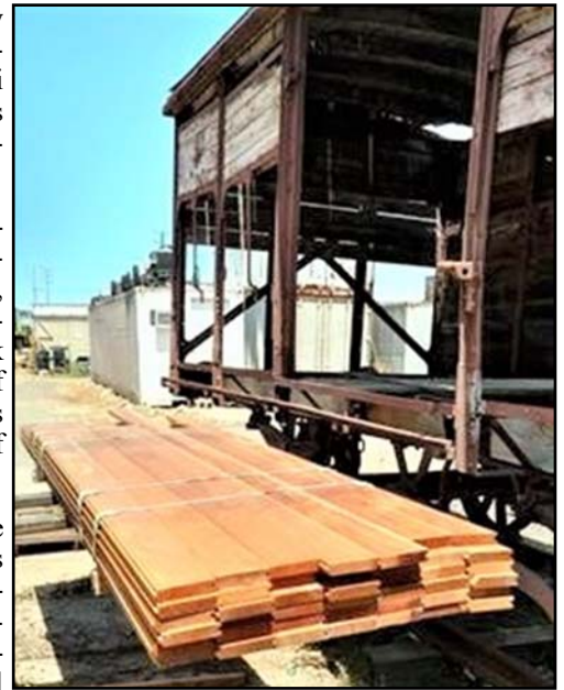
Hawaii Boxcar in background and new tongue & groove boards have been milled to duplicate the original boards.
